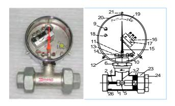
**Installation:** Installation horizontal wherever possible on the basis of shematic 1, 2 or 3, only pressure line, not suction side since the seal of the control shaft 5) is not vaccum-tight. However, the monitor may be subject to temporary depressurization. It is also possible to install the monitor in a vertikal line with rising or falling flow, please refer to shematics 3 and 4.
