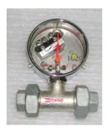
With flow monitor and scale are models of a novel design, operating on the slinding spool-principle; they are also suitable for extremely low flow rates of pure, neutral media such as water, oil or air and temperatures up to 80° degrees, or line pressure 0 -10/16 bars. Temporary depressurisation is not disadvantegeous.
